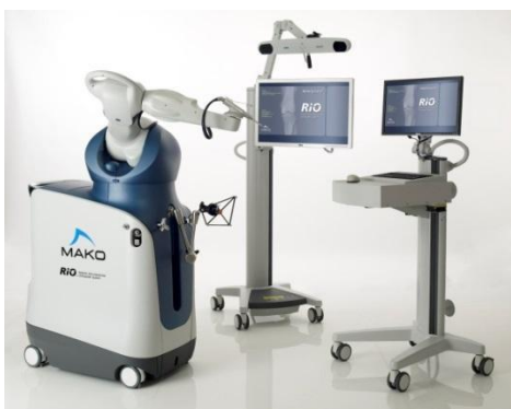
Mako Robotic arm and guiding system
